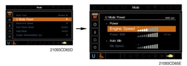
Engine Step Idle speed speed shift (rpm) **( | )** (rpm) (bar) 1000 (low idle) 1500 0 2 1050 1550 3 3 1600 1100 (decel rpm) 6 4 1650 1150 9 5 1700 1200 12 1750 1250 6 16 7 1800 1300 20 8 1850 1350 26 9 1900 1400 32
