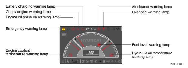
Each warning lamp on the top of the LCD pops up on the center of LCD and the buzzer sounds
