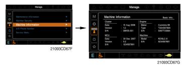
· This can confirm the identification of the cluster, MCU, engine and machine.
